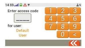
**The login screen** for particular Users authorised to operate the alarming unit by means of a touch panel.
