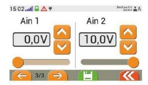
**The Outputs** Menu is used to configure the status of alarm outputs and adjust the values of voltage for the analogue 0..10V outputs.
