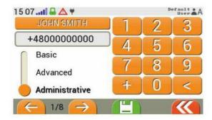
The SIM Access Menu enables to enter Users data together with the level of privileges for communication with the alarming unit by means of GSM (up to 8 Users).
