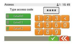
The 'Access' screen is used to unlock the following access levels for flock's settings as well as controller's settings.
