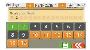
It is possible to assign scales pans and sensors to the flock in an intuitive and clear way: devices already assigned are marked with green colour, unavailable devices (assigned to other flocks) are marked with dark grey colour while available devices with orange colour.
