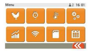
From the basic screen, after unlocking the access of 'Level 1', it is possible to move to the menu of settings. Particular groups of settings are illustrated as 'tiles'.
