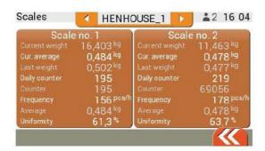
The 'Scales pans' screen shows the current indications gained from weighing acts on particular scales pans that have been assigned to the flock.
