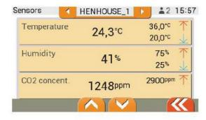
The 'Sensors' screen is used to preview indications from the sensor (single or multiparameter) assigned to the flock and settings of alarm thresholds for particular parameters (if the sensor's mode is adjusted as 'alarming').
