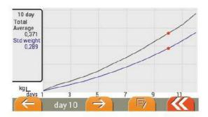
The 'Statistics' screen allows for graphic illustration of data from weighing acts by means of charts. There is presented a chart of the average weight (red colour) in comparison to the standard one (grey colour).
