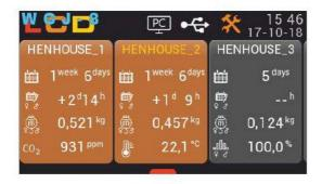
The 'basic screen' enables a fast preview of selected by the User parameters of weighing for each of the flocks and the status of system operation. By pressing the field of the flock it is possible to move to its detailed view.
